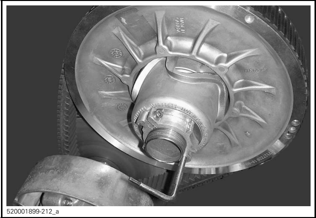
TYPICAL - PULLEY EXPANDER INSTALLED ON ADJUSTER HUB
