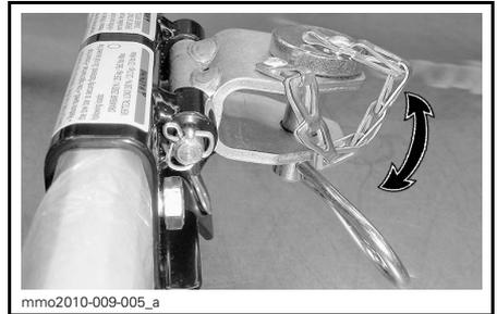
**HITCH MOVES FREELY WHEN TOWING**
