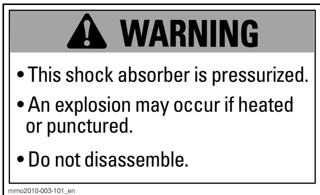
LABEL 11 - ON SHOCK GAS CHARGED ABSORBERS
