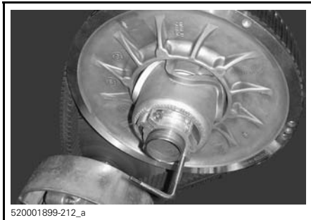
TYPICAL - PULLEY EXPANDER INSTALLED ON ADJUSTER HUB
