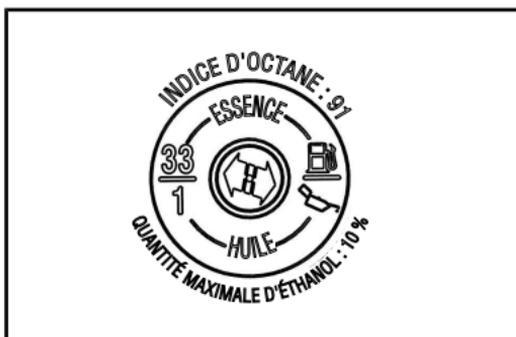
*SUR LE BOUCHON DU RÉSERVOIR DE CARBURANT (DANS LES PAYS UTILISANT DES INDICES D'OCTANE AKI (RON+MON)/2 AFFICHÉS À LA POMPE)*
