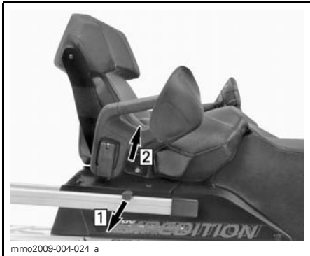
Step 1: Pull rubber tab Step 2: Lift RH side
