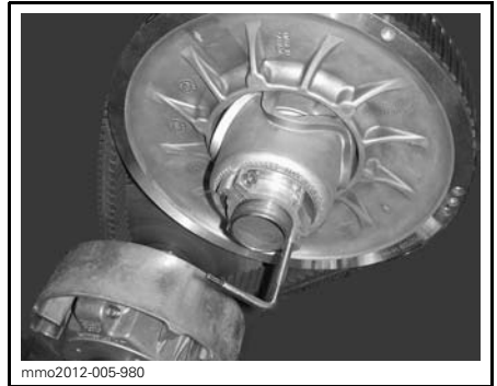
PULLEY EXPANDER ON ADJUSTER HUB
