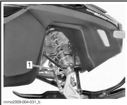
TYPICAL - CAM TYPE PRELOAD
