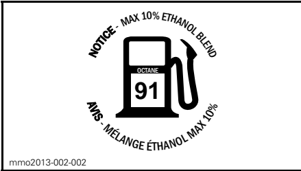
LOCATED ON FUEL CAP - IN COUNTRIES USING PUMP POSTED AKI (RON+MON)/2 OCTANE RATINGS
