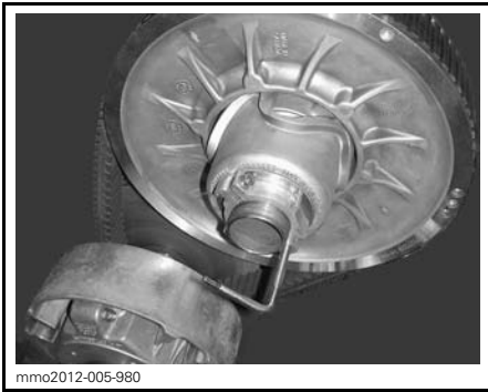
PULLEY EXPANDER INSTALLED ON ADJUSTER HUB
