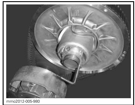
PULLEY EXPANDER INSTALLED ON ADJUSTER HUB
