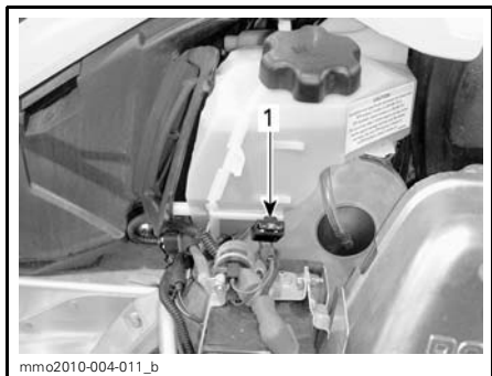
1. Fusible principal (30 A)
