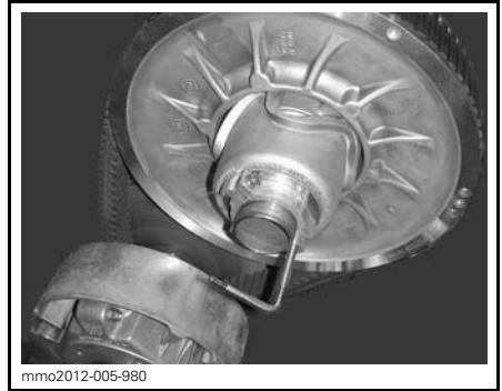
PULLEY EXPANDER INSTALLED ON ADJUSTER HUB
