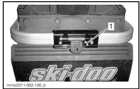
mm02011-002-100_b HITCH (TONGUE TYPE) 1. Tongue
