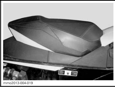
TYPICAL - SEAT INSTALLED
