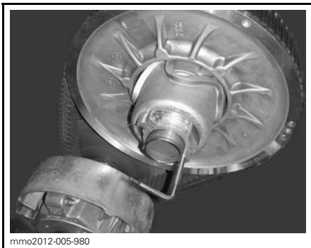
PULLEY EXPANDER INSTALLED ON ADJUSTER HUB
