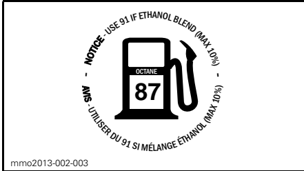
LOCATED ON FUEL CAP - ON 550F AND 600 ACE ENGINES (IN COUNTRIES USING PUMP POSTED AKI (RON+MON)/2 OCTANE RATINGS)
