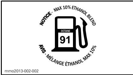
LOCATED ON FUEL CAP - ON 600 HO E-TEC ENGINE (IN COUNTRIES USING PUMP POSTED AKI (RON+MON)/2 OCTANE RATINGS)
