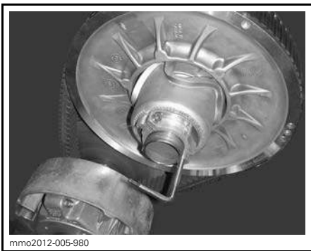
PULLEY EXPANDER INSTALLED ON ADJUSTER HUB
