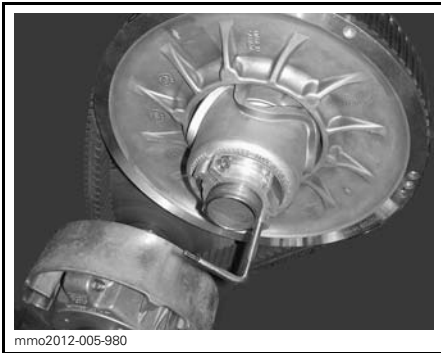
PULLEY EXPANDER INSTALLED ON ADJUSTER HUB
