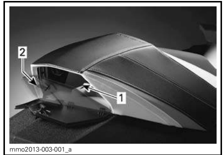
mmo2013-003-001_a 1. Storage compartment 2. Latch
