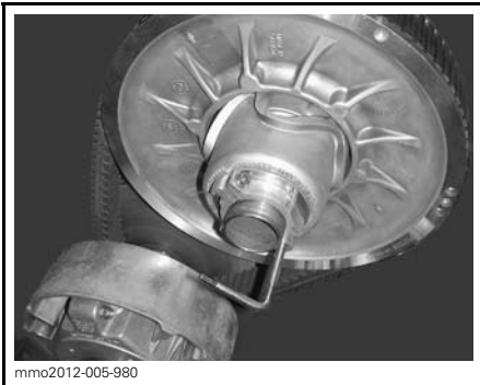
PULLEY EXPANDER INSTALLED ON ADJUSTER HUB
