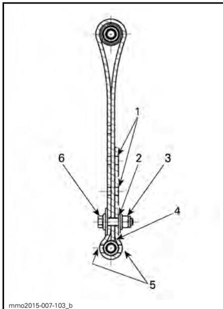
**POSITION DE LA COURROIE D'ARRÊT (COURTE)**
