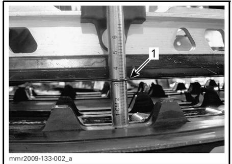
1. Deflection O-ring aligned with slider shoe
