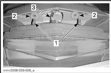
1. Taillight housing retaining pins
