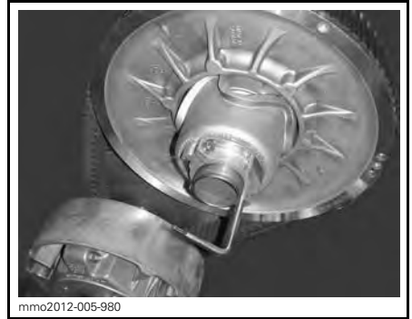
mmo2012-005-980 PULLEY EXPANDER INSTALLED ON ADJUSTER HUB
