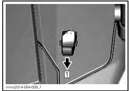
TYPICAL Step 1: Press bottom end of switch
