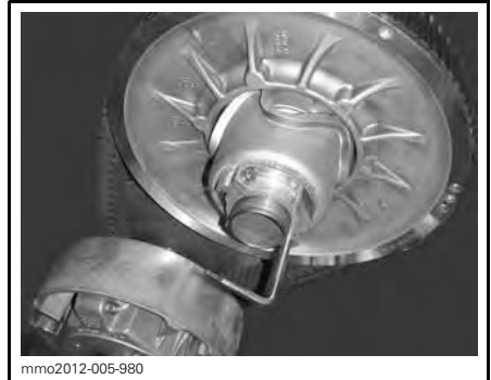
PULLEY EXPANDER INSTALLED ON ADJUSTER HUB
