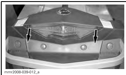
TYPICAL - CAREFULLY PULL OUT AT CORNERS
