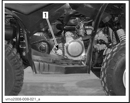
TYPICAL — RH SIDE OF ENGINE 1. Dipstick
