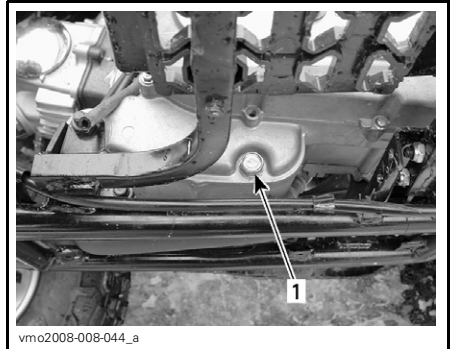
LH SIDE OF ENGINE 1. Drain plug
