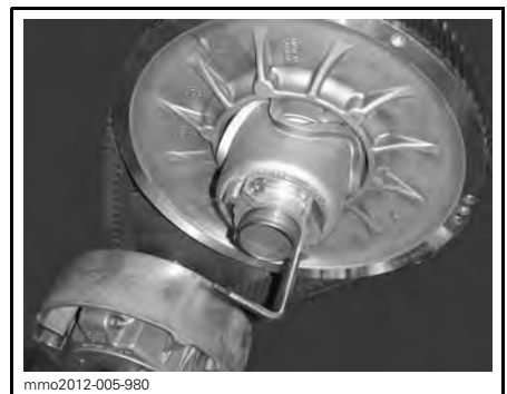
PULLEY EXPANDER INSTALLED ON ADJUSTER HUB
