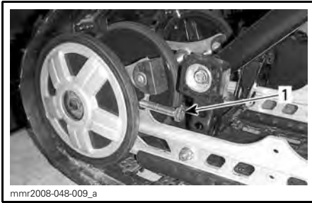
1. RH adjustment screw
