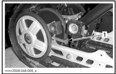
1. RH adjustment screw
