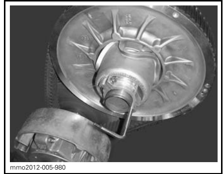
mmo2012-005-980 PULLEY EXPANDER INSTALLED ON ADJUSTER HUB
