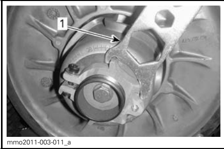
1. Suspension adjustment tool
