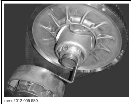
PULLEY EXPANDER INSTALLED ON ADJUSTER HUB
