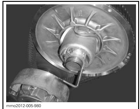
PULLEY EXPANDER INSTALLED ON ADJUSTER HUB
