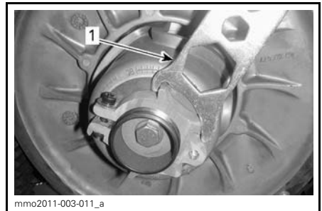
ALUMINUM ADJUSTER HUB 1. Suspension adjustment tool
