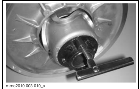
PULLEY EXPANDER ON PLASTIC ADJUSTER HUB
