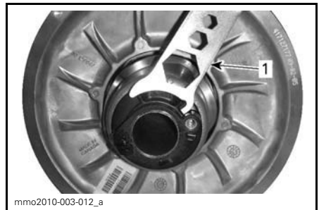
PLASTIC ADJUSTER HUB 1. Suspension adjustment tool
