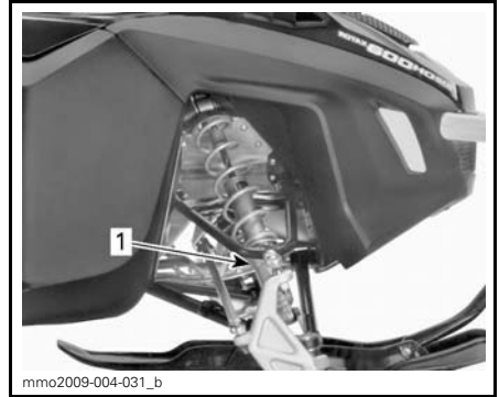
TYPICAL - CAM TYPE PRELOAD 1. Adjustment cam
