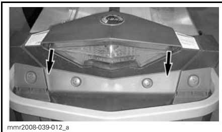
TYPICAL - CAREFULLY PULL OUT AT CORNERS
