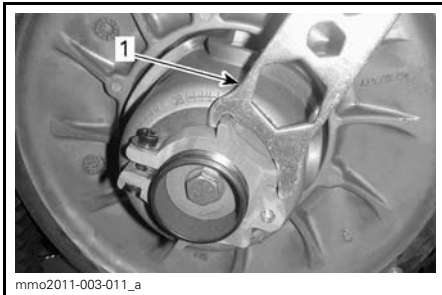
TYPICAL - PRELIMINARY SETTING 1. Lowest portion of cogs even with external surface of drive belt
