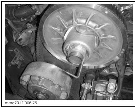
PULLEY EXPANDER INSTALLED ON ADJUSTER HUB
