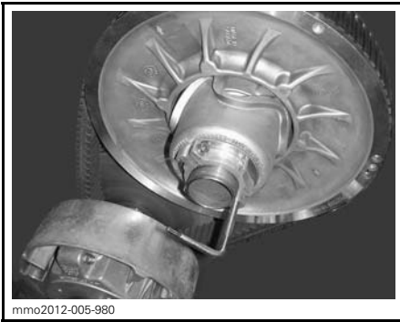
PULLEY EXPANDER INSTALLED ON ADJUSTER HUB
