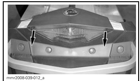
TYPICAL - CAREFULLY PULL OUT AT CORNERS
