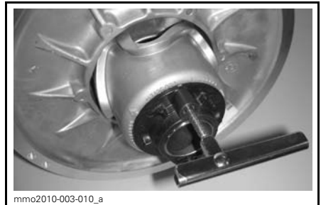
PULLEY EXPANDER ON PLASTIC ADJUSTER HUB
