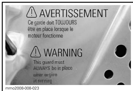
ON BRAKE DISC GUARD (BARE METAL TUNNEL)
