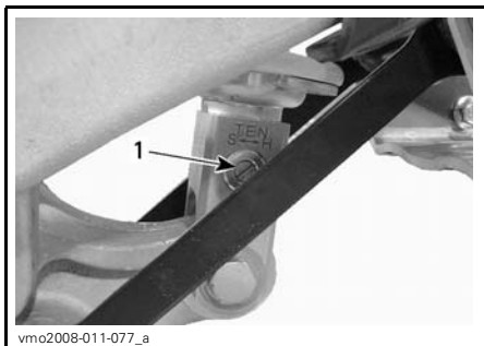
1. Rebound adjuster (flat screwdriver)
