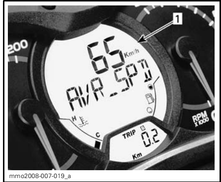
MULTIFUNCTION ANALOG/DIGITAL GAUGE 1. Multifunction display
