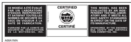
Other important labels on the vehicle are WARNING or CAUTION labels relating to safety, maintenance and/or snowmobile operation. Ensure all such labeling is retained on the vehicle and its content is followed by vehicle operator.
