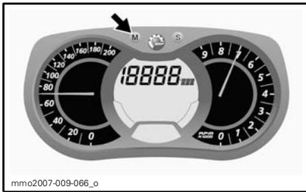
To reset maximum temperature recorded, push the MODE (M) to select mode.
