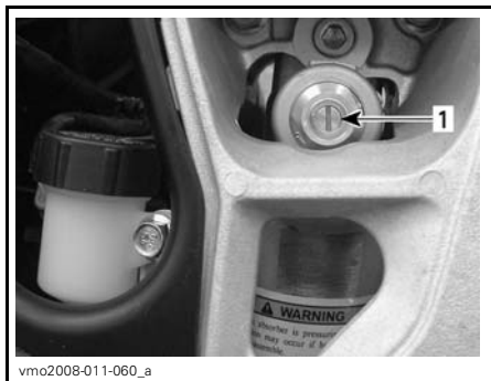
1. Compression adjuster (flat screwdriver)
