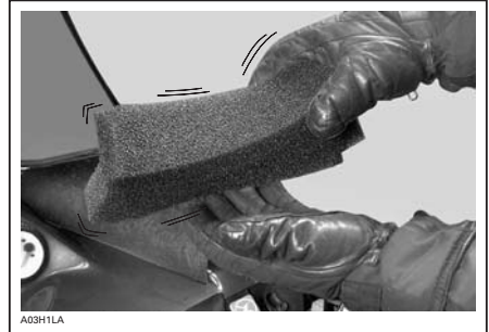
TYPICAL — SHAKING SNOW FROM FILTER
