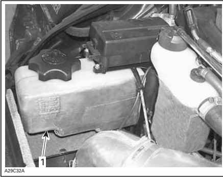
1. Injection oil reservoir
