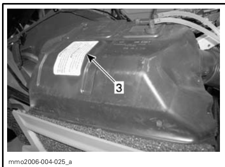
mmo2006-004-025_a AIR INTAKE SILENCER (BODY SIDE) — FAN-COOLED
