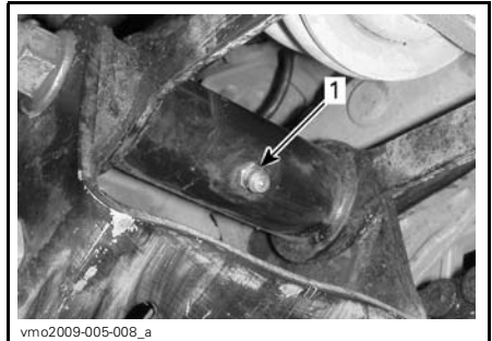
PIVOT ARM 1. Grease fitting
