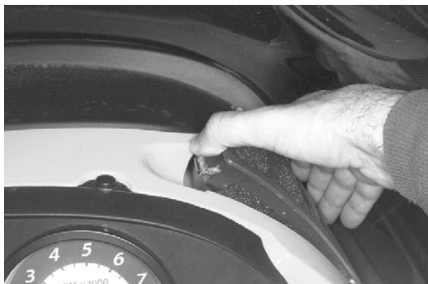
REMOVAL OF RIGHT SIDE PRIMARY FILTER GRILL
