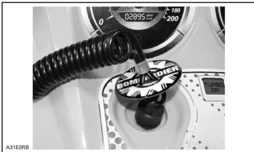
*TETHER CORD CAP INSTALLED ON POST*
