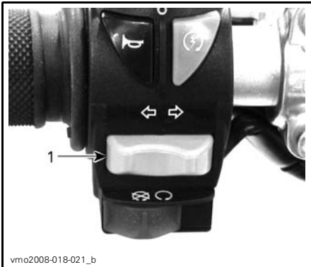
1. Turn signal switch
