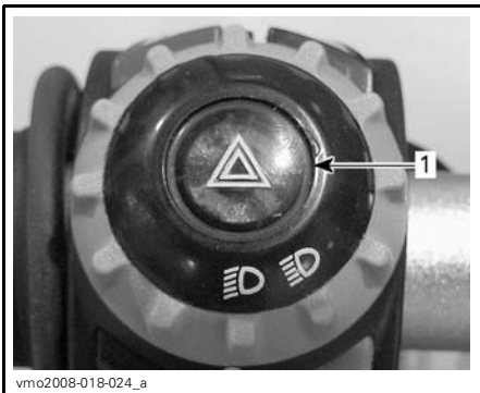
1. Hazard warning indicator light
