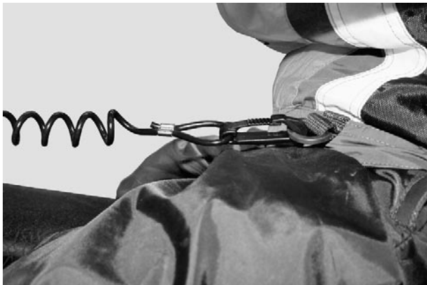
TETHER CORD ATTACHED TO CLOTHING EYELET
