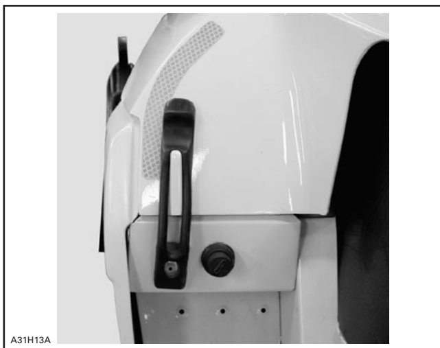
LEFT SIDE SHOWN — HOOD LATCH IN FASTENING POSITION
