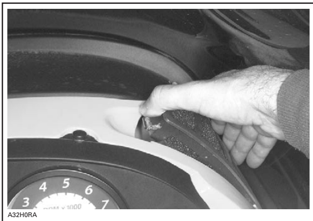
REMOVAL OF RIGHT SIDE PRIMARY FILTER GRILL
