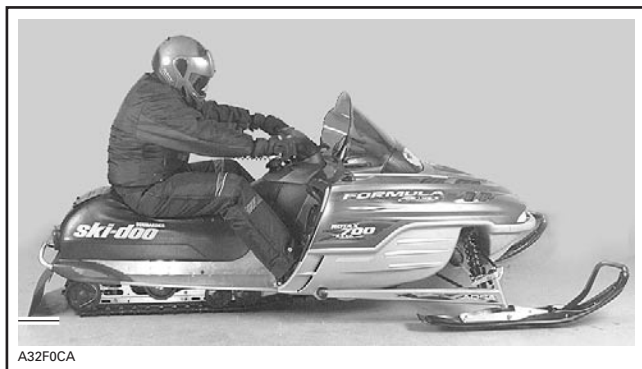
TYPICAL — TOO SOFT OF ADJUSTMENT
