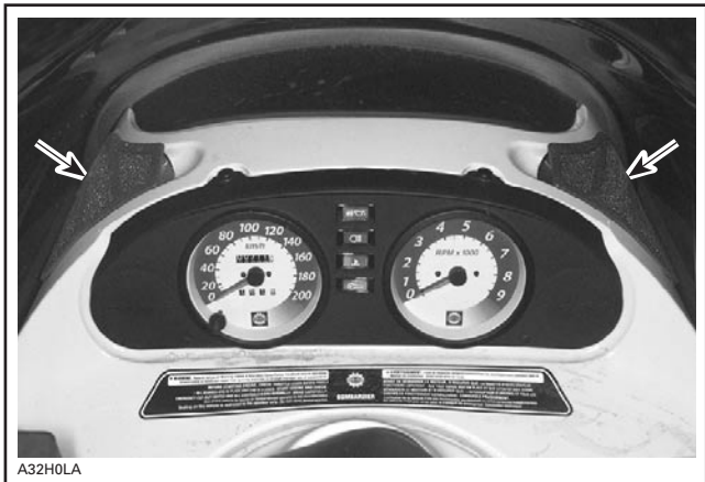
TYPICAL — PRIMARY FILTER LOCATION
