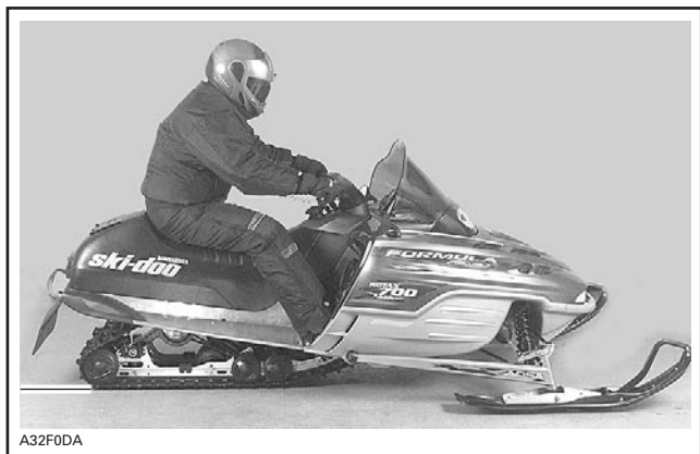
TYPICAL — TOO HARD OF ADJUSTMENT
