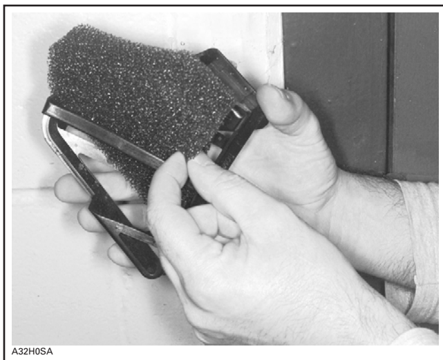
REMOVAL OF FILTER FROM ITS GRILL
