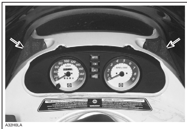
PRIMARY FILTER LOCATION
