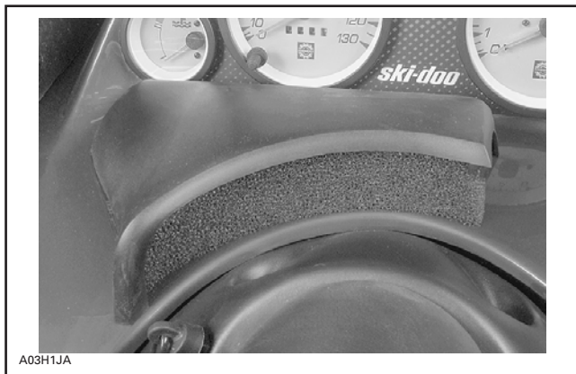
TYPICAL — FILTER INSTALLED
