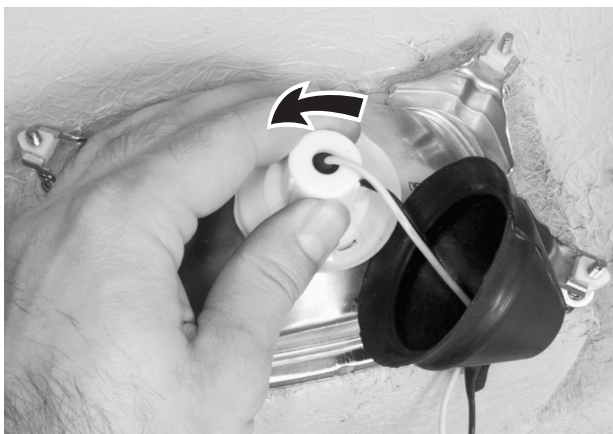
RUBBER BOOT AND BULB RETAINER REMOVAL
