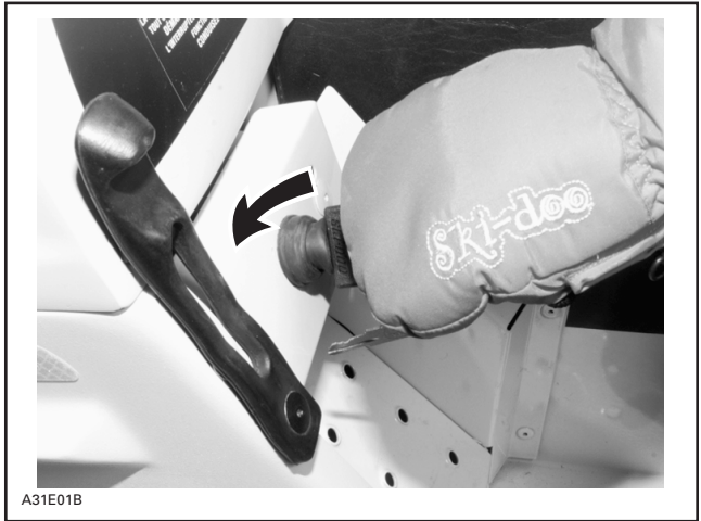
TURNING IGNITION KEY TO STOP ENGINE
