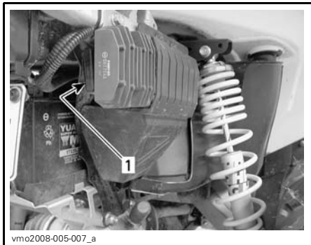
TYPICAL — REAR FUSES LOCATION 1. Fuses holder
