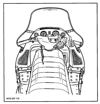
**Steering** - The steering handlebar assembly controls the direction of travel of the snowmobile. As the handlebar is rotated to right or left, the skis are turned in the direction of intended travel. Proper shifting of your body weight helps in turning. Occasionally check your steering system to be sure its movement is unrestricted.
