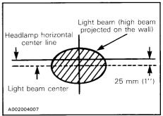
To adjust, remove the four caps, turn upper or lower adjusting screws to obtain desired beam position.
