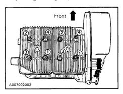
**IMPORTANT:** The engine head nut torque should be checked after the first 5 hours of operation.
