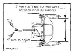
The illustration below showns a crosssection of the skis and where to measure for toe-out adjustment.
