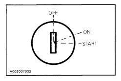
Key, operated, 3 position switch. To start engine, turn key to START position and hold. Return key to ON position immediately when engine has started. To stop engine, turn key to OFF position.
