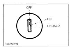
Key operated, 3 position switch. To start the engine, first turn the key to ON position. To stop the engine, turn the key to OFF position.
