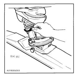
Reinstall boot and secure the spring.
