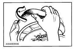
5. Slip the belt out from the drive pulley and remove completely from vehicle.
