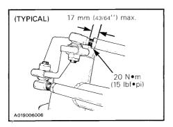
WARNING: The ball joint socket must run parallel with the steering arm. The socket must be restrained when tightening the tie rod end lock nuts.
