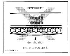
CAUTION: Do not force or use tools to pry the belt into place, as this could cut or break the cords in the belt.
