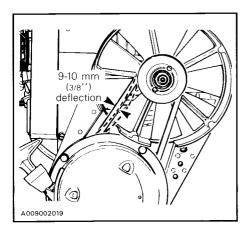
If belt seems damaged or if tension is incorrect, contact an authorized dealer immediately.
