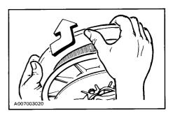
4. Slip slackened belt over the top edge of the sliding half.
