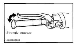
After the adjustment, brake should apply fully when lever is approximatively 13 mm (1/2") from handlebar grip. If not, do not tamper with the brake, contact the dealer.
