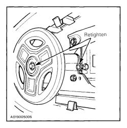
Restart engine, rotate track **slowly** and recheck alignment.
