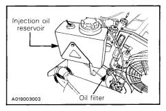
CAUTION: An obstructed injection oil filter will cause oil starvation resulting in serious engine damage.
