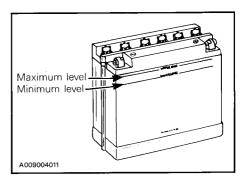
If necessary add distilled water. Battery connections must also be free of corrosion. If cleaning is necessary remove corrosion using a stiff brush then clean with a solution of baking soda and water. Rinse and dry well.
