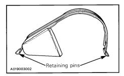
3. Lift and remove the belt guard assembly.
