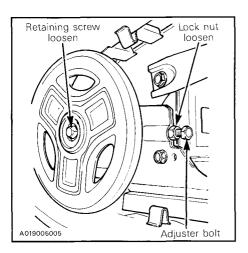
NOTE: Track tension and alignment are inter-related. Do not adjust one without the other.
