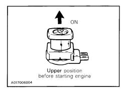
Ensure the tether cut-out cap is in position and that the cord is attached to the clothing.
