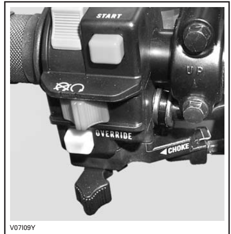
CHOKE LEVER IN THE FULL CHOKE POSITION
